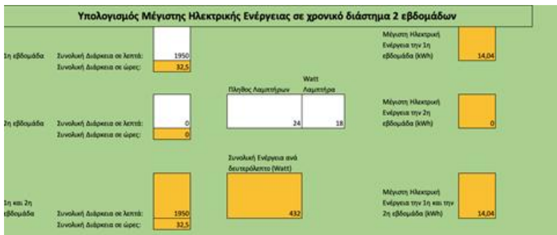
Figure 35 Verification of energy consumption calculations using the Excel file "CalkWh" - the comparison interval.
